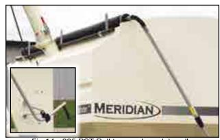
Fig 14 - 225 RST Roll tarp and crank handle
