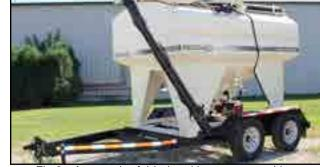
Fig 9 - Auger tube folded and in storage position
