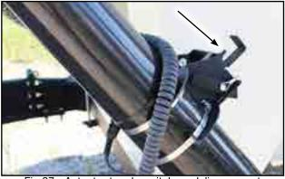
Fig 37 - Actuator toggle switch on delivery spout
