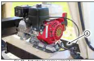
Fig 43 - Actuator to engine wiring harness
