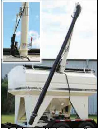
Fig 10 - Auger tube unfolded into working position
