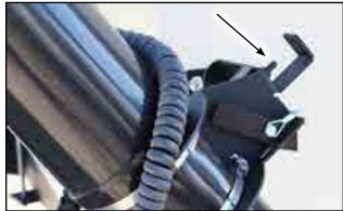
Fig 11 - Actuator toggle switch on delivery spout
