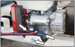
Fig 49 - Engine mounting bolts
