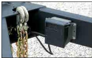
Fig 16 - Break-Away system control box
