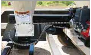
Fig 51 - Drive belt routing
