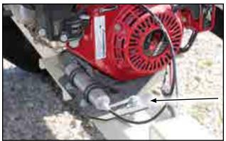
Fig 50 - Engine base stabilizing bolt
