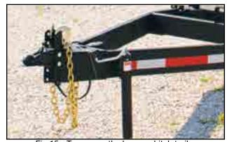
Fig 15 - Tongue on the bumper hitch trailer
