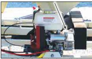
Fig 7 - Centrifugal clutch and auger drive belt
