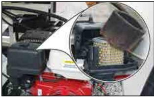
Fig 39 - Engine air filter
