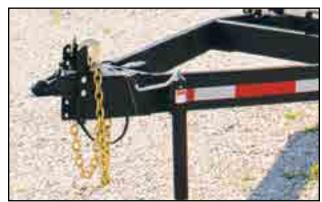
Fig 21 - Trailer hitch with safety chains
