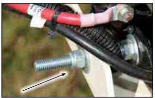
Fig 47 - Engine base adjustment bolt
