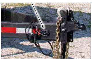
Fig 53 - Break-Away cable on hitch tongue
