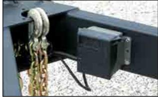
Fig 52 - Break-Away system control box
