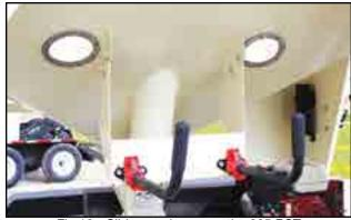
Fig 12 - Slide gate levers on the 225 RST
