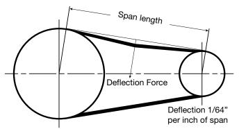
Fig 48 - Tension calculation
