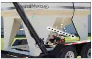
Fig 8 - Battery in corner of frame
