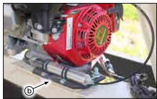
Fig 44 - Actuator bolts
