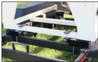
Fig 19 - Load cells between tender and trailer frame
