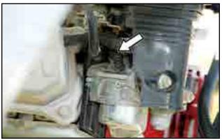
Fig 42 - Engine speed setscrew
